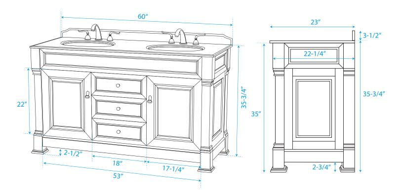
\*Note: Due to high probability of breakage, the backsplash comes in two pieces, cut from same piece. All Measurements are  $\pm 1/4$ .
